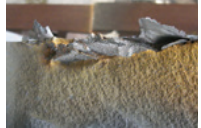
Ziehschrittüberlappung an einem Stangenende
